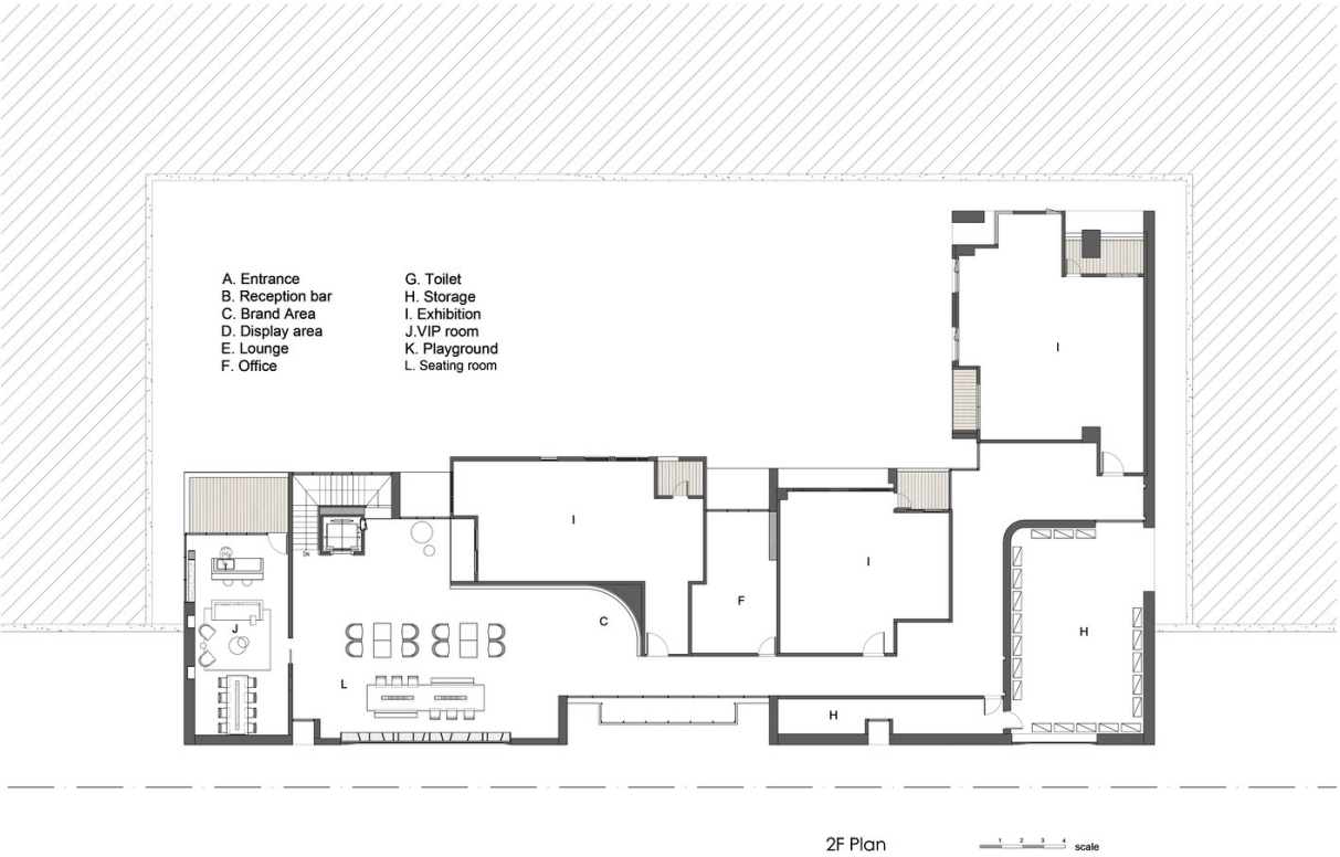
Fig. 9: Second floor plan.
